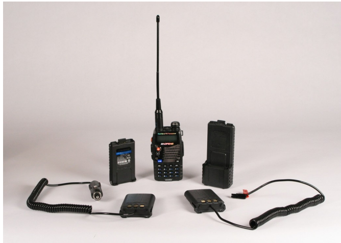
Rechargeable battery, AA Pack, Cigaret Lighter, and power poles all as power methods
